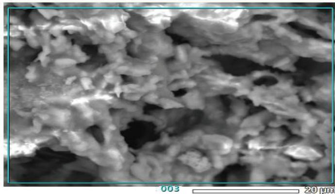
FIGURE 6. Porous microstructure of activated carbon with 15% composition
