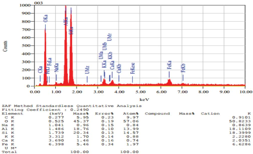
FIGURE 7. Analysis of porous ceramic elements on 15% activated carbon composition
