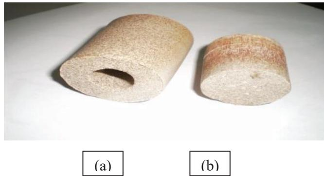
FIGURE 1. Porous ceramic sample (a) hollow cylinder, (b) pellet cylinder
