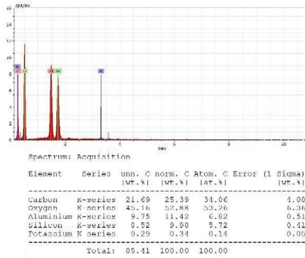
**FIGURE 2.** Analysis of Kaolin Sample Elements
