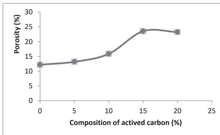
FIGURE 4. Relation between Porosity and Activated Carbon
