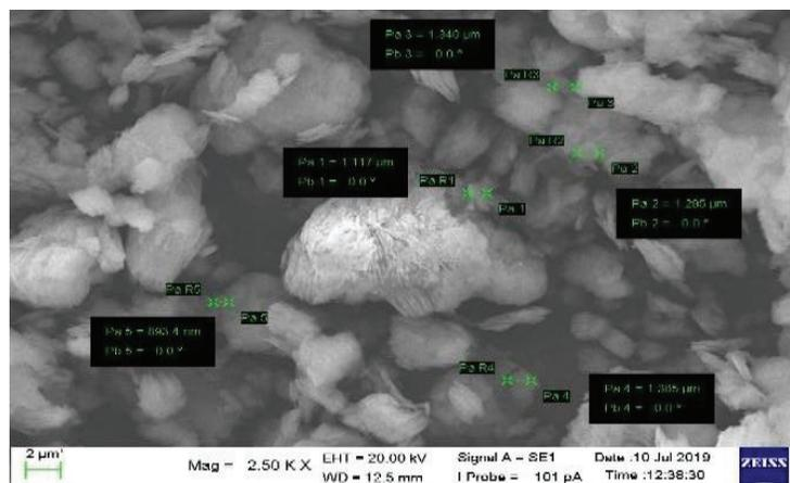
FIGURE 3. Kaolin Microstructure
