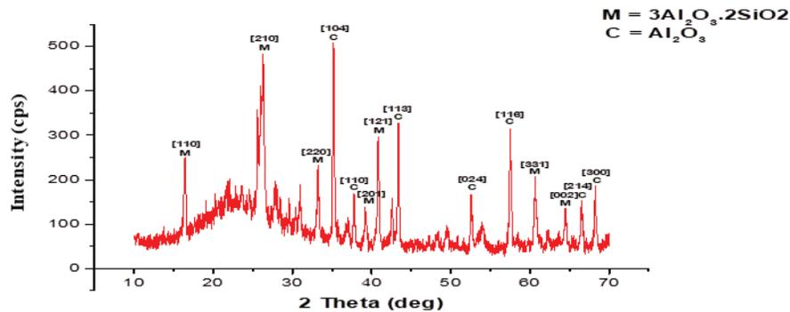
FIGURE 5. Porous ceramic diffraction pattern on 15% activated carbon composition
