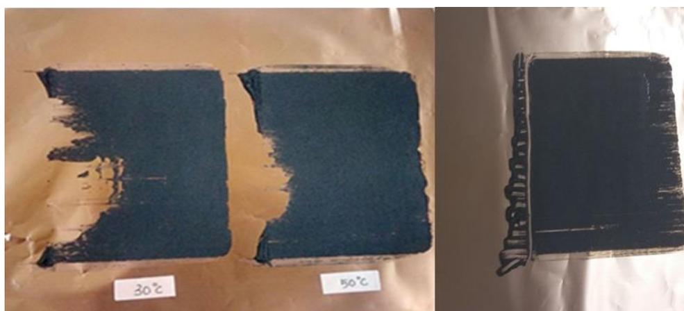
**Figure 2.** LTO sheets with PTFE binder with the different heating process.
