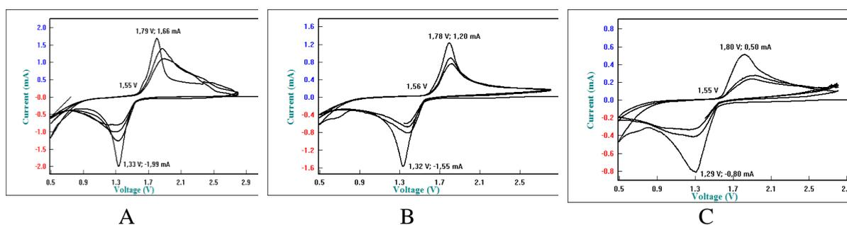
**Figure 4.** Cyclic voltammograms of LTO using PTFE binders with varying heating temperature (A). 30 °C, (B) 50 °C, and 70 °C
