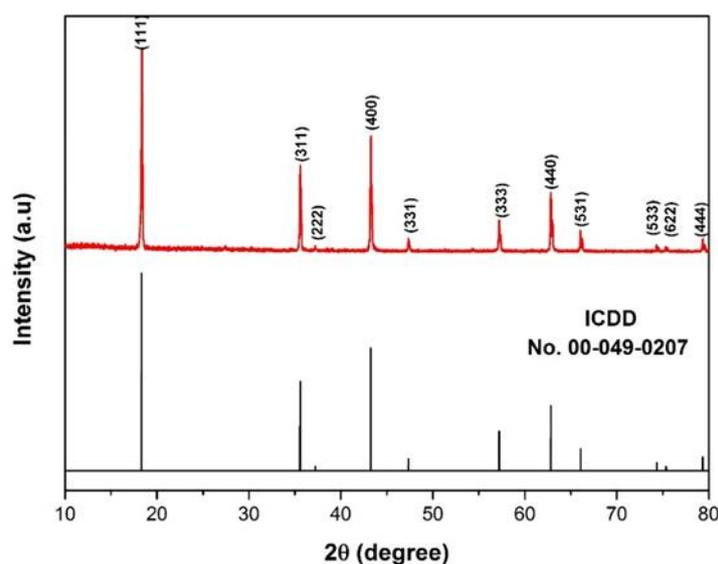
**Figure 1.** XRD pattern of LTO powder synthesized via solid-state reaction
