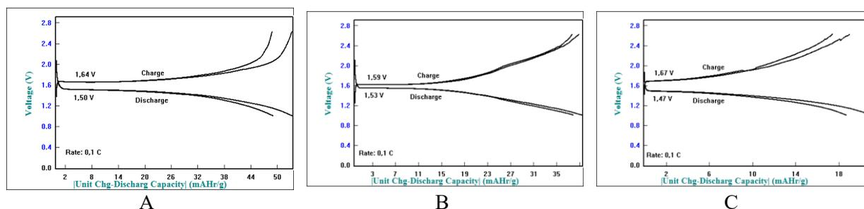
**Figure 5.** Galvanostatic charge and discharge curve of  $Li_4Ti_5O_{12}$ .
