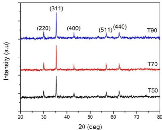
**Figure 1.** XRD diffraction pattern of MgFe<sub>2</sub>O<sub>4</sub>.
