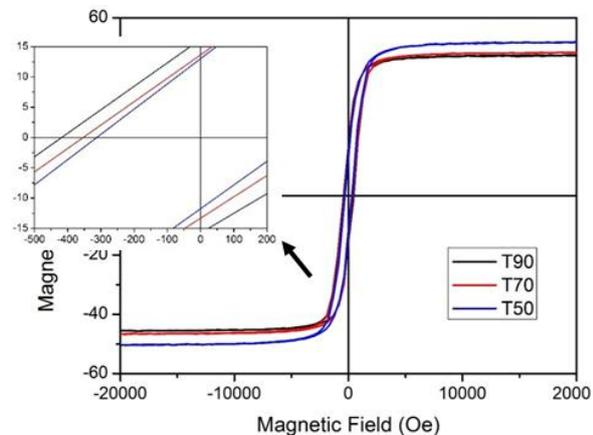
**Figure 2.** Hysteresis curves of MgFe<sub>2</sub>O<sub>4</sub>.
