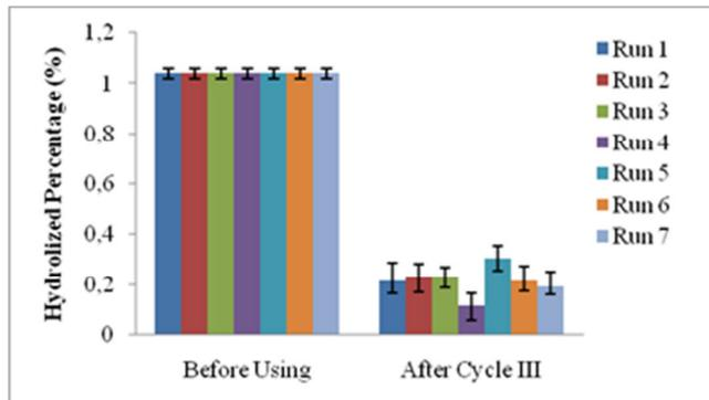
**Fig. 7. Diagram of Lipase activities by *Lipozyme RM IM* before using and after recycle III.**
