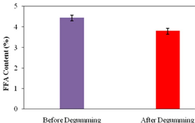
Fig. 2. Content of FFA of CPO before and after degumming.
