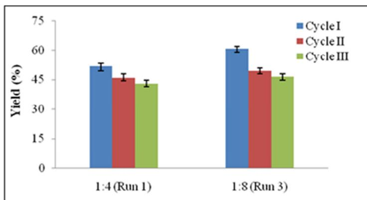
Fig. 5. Effect of reactant molar ratio to the decreasing of biodiesel caused by recycling of *Lipozyme RM IM* in temperature 45°C.
