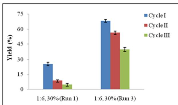
**Fig 6. Effect of *Lipozyme RM IM* to the decreasing of yield caused by recycling of *Lipozyme RM IM*.**
