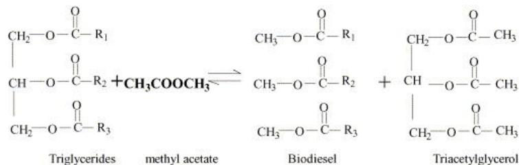
**Fig. 1. Interesterification reaction of Triglyceride with Methyl Acetate.**
