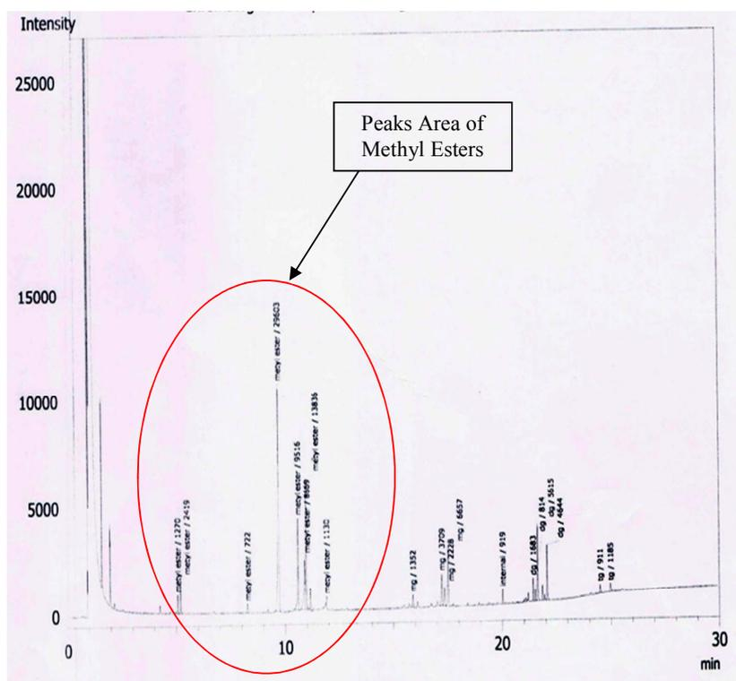
**Fig. B-1. Chromatogram of Biodiesel Yield (Run 5).**
