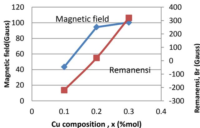
Figure 5. The relationship between magnetic field strength and remanence, Br<sup>[13]</sup>.
