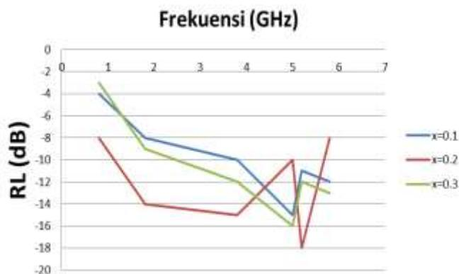
Figure 3. Reflection Loss of  $\text{BaFe}_{12-x}\text{Cu}_x\text{O}_{19}$  <sup>[13]</sup>
