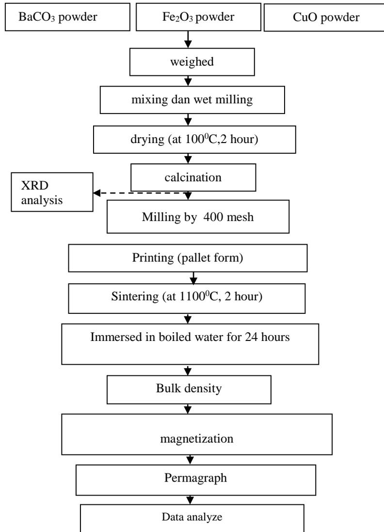
Figure 1. Flowchart of (BaFe<sub>12-x</sub>Cu<sub>x</sub>O<sub>19</sub>) preparation and characterization
