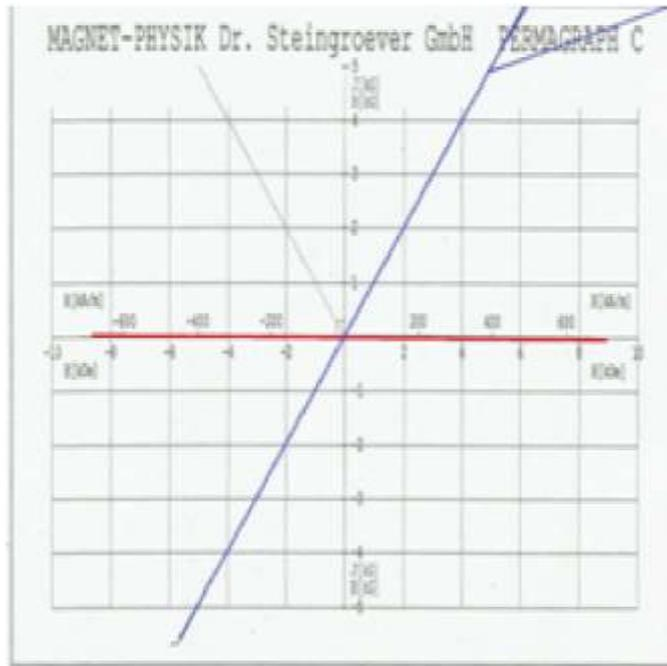
Figure 2. Permagraph result of  $\text{BaFe}_{12-x}\text{Cu}_x\text{O}_{19}$  <sup>[13]</sup>
