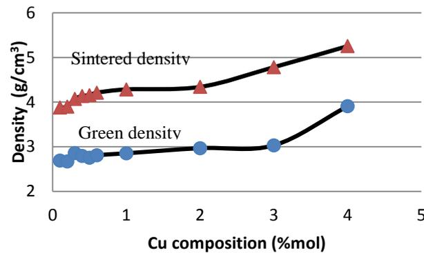
Figure 4. Relationship between density before and after sintering with Cu composition (%mol)<sup>[13]</sup>.
