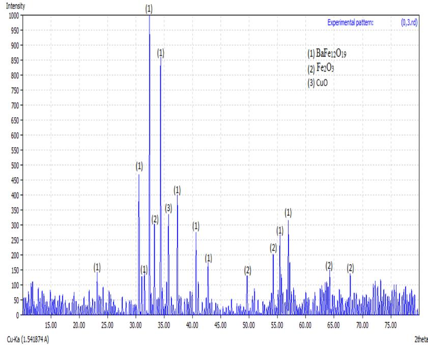
Figure 7. XRD patterns of BaFe<sub>12</sub>O<sub>19</sub> <sup>[13]</sup>.
