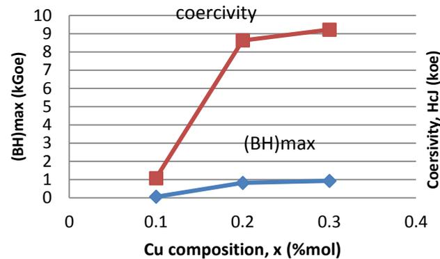
Figure 6. The relationship between (BHmax) and (HcJ) on Cu composition (%mol)<sup>[13]</sup>.
